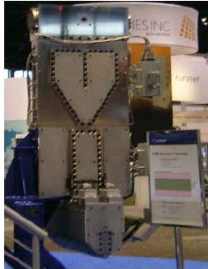
Feed-block/dies for producing 514 layered film (Cloeren, NPE 2009)
