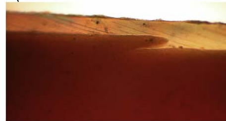
Fig. 6-29 Cross-section of wave-like melt disturbance of core layer entering the skin layer.
